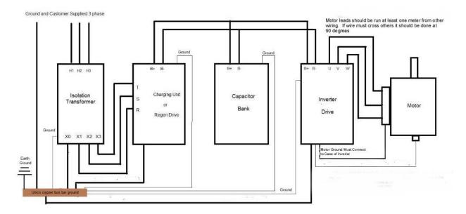
It is important that all high power leads be run in their own conduits, at least one meter away from other conductors. Any crossings of wires should be done at 90 degrees. It is important that the motor ground be terminated at the chassis of the inverter. From there, a connection to bus should be made. But there should not be a direct connection between the motor and the bus bar.
