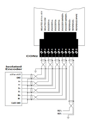
While the power component and encoder grounds tend to be the most important, proper grounding is important elsewhere. Please refer to the Unico 2400 or 1100 manual for recommendations for grounding of other connections.
