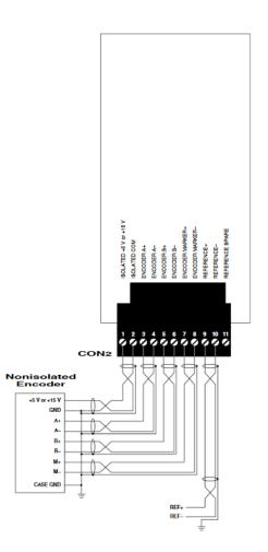
With a non insulated encoder, the shield and chassis of the encoder are grounded at the encoder. There are no chassis or earth grounds at the DSP encoder interface.
