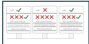
In rare instances, IGBT failure may transmit high voltage into drive control circuits and cascade to other drives and logic circuits.
