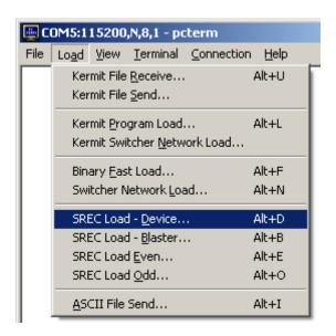
To load an EPROM file to a S4000 processor, connect the PC to the S4000 device through the serial port. Make sure the baud rate in PCTerm is set to be the same as the one the device is expecting. Get the device ready for a file transfer. By selecting **SREC Load** – **Blaster...**, the standard file dialog is opened prompting the user for the EPROM program file. Once the file is selected, the following dialog is displayed indicating
