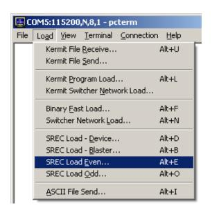
To load an EPROM file to an EPROM blaster, connect the PC to the blaster through the serial port. Make sure the baud rate in PCTerm is set to be the same as the one the blaster is expecting. Get the blaster ready for a file transfer. By selecting **SREC Load** – **Even...**, the standard file dialog is opened prompting the user for the EPROM program file. Once the file is selected, the following dialog is displayed indicating PCTerm is
