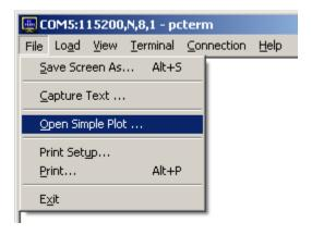
PCTerm also supports a graphing function that plots the contents of the file obtained during data upload called Simple Plot. Upon selecting **Open Simple Plot...**in the menu, the user is requested to select a file containing the data sample that was previously uploaded from a UNICO Series 4000 device. Once the appropriate file is selected, a new window appears containing a graph for each channel contained in the sample. The following is an example of a data sample.
