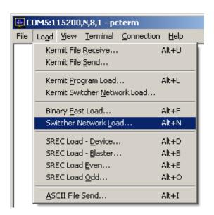
Selecting **Switcher Network Load...** from the menu opens the standard file dialog box prompting the user for the UNICO S4000 program file to send. These files have the \*.l extension. Once the file is selected, click the "Open" button to begin transmission of the file through Kermit. While transmission is in progress, PCTerm provides a dialog
