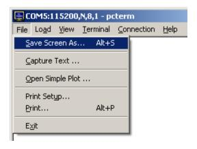
This feature saves the contents of the current screen to a text file. The standard file dialog appears and prompts the user for the file to save the screen text to. Alternatively, the 'Alt + S' key sequence may also be typed to perform this function.
