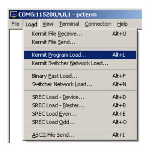
Selecting **Kermit Program Load...** from the menu opens the standard file dialog box prompting the user for the UNICO S4000 program file to send. These files have the \*.l extension. Once the file is selected, click the "Open" button to begin transmission of the file through Kermit. While transmission is in progress, PCTerm provides a dialog window that reports on the status of the transaction as shown below. Alternatively, the key sequence Alt + L will also perform this function.
