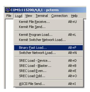
Selecting **Binary Fast Load...** from the menu opens the standard file dialog box prompting the user for the UNICO S4000 program file to send. These files have the \*.l extension. Once the file is selected, click the "Open" button to begin transmission of the
