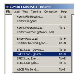
To load an EPROM file to an EPROM blaster, connect the PC to the blaster through the serial port. Make sure the baud rate in PCTerm is set to be the same as the one the blaster is expecting. Get the blaster ready for a file transfer. By selecting **SREC Load** – **Blaster...**, the standard file dialog is opened prompting the user for the EPROM program file. Once the file is selected, the following dialog is displayed indicating PCTerm is
