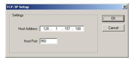
The dialog above can be used to configure a TCP/IP connection. A valid IP address must be specified for the **Host Address** field in the form: xxx.xxx.xxx.xxx. The **Host Port** field specifies which port on the specified host to connect to. When a connection is established through TCP/IP, the title bar of the application displays both the host IP address and port.
