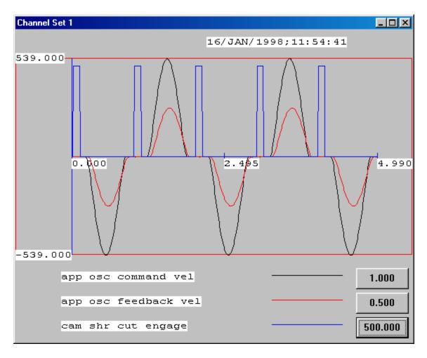
Each channel is displayed with a different color. The time and data recorded at the time of sampling are also printed at the top of the graph as an identifying feature. This time stamp is stored within the sample file for archiving purposes.
