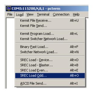
To load an EPROM file to an EPROM blaster, connect the PC to the blaster through the serial port. Make sure the baud rate in PCTerm is set to be the same as the one the blaster is expecting. Get the blaster ready for a file transfer. By selecting **SREC Load** – **Odd...**, the standard file dialog is opened prompting the user for the EPROM program file. Once the file is selected, the following dialog is displayed indicating PCTerm is
